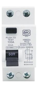
In the event of an Earth Fault in the installation or the operation of the test button, the dolly will move to the OFF position.
